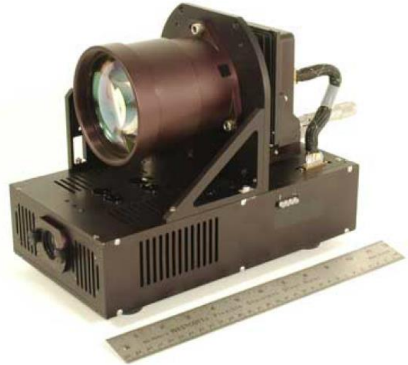
Figure 3 – Flash Laser Radar (LADAR) manufactured by Advanced Scientific Concepts of Santa Barbara California. The lower portion is a custom-developed 10 milliJoule class 1.54 \mu\text{m} laser illuminator. The actual camera is quite small, located directly behind the optical lens.
