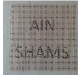
Fig. 10: Fabricated proposed HIS.
