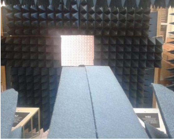
Fig. 13: Measurement setup of S_{11} .
